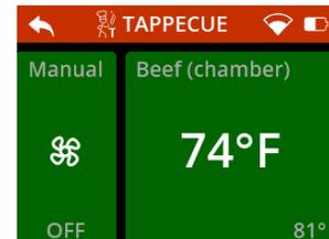
You can adjust the Set Temp from your app at any time. From the App, go to the Current Session, the Select Tappecue, then Temperatures, then slide over until the probe port with Cruise Set Points and edit with the pencil the Max Temp. This will be a way to turn the blower off or on manually.
