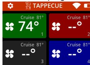
You can manually turn off the fan by pressing the touch screen on the fan, it will switch from AUTO, to MANUAL ON or MANUAL OFF by touching the left hand pane. We have found this is convenient for turning off the FAN while raising the lid or door. Then turning back on when shutting the door.
